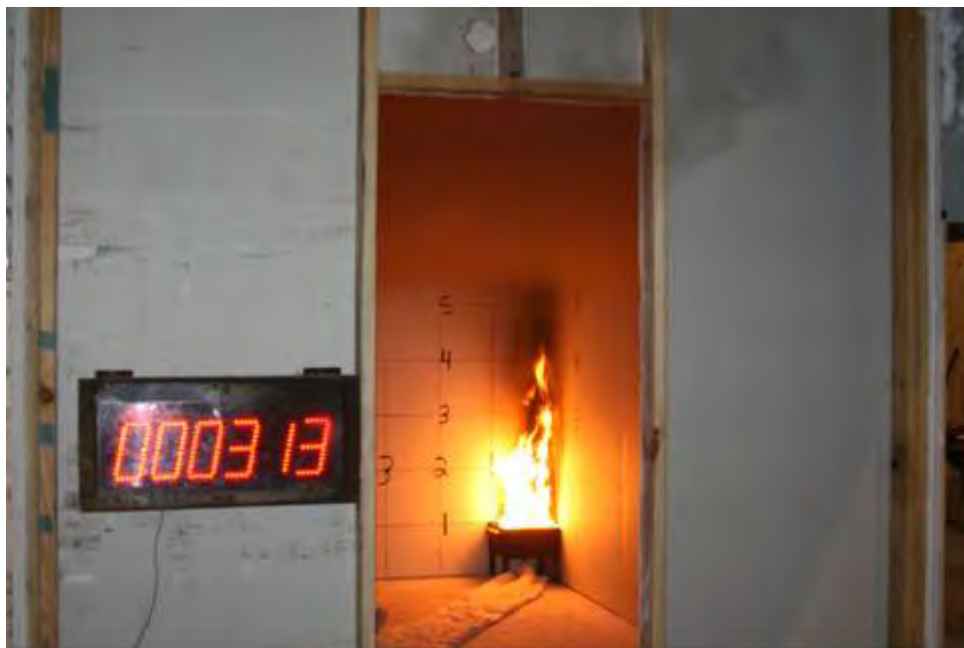
Figure 2. Burner at 40 kW: 3 min 13 s into Test.
