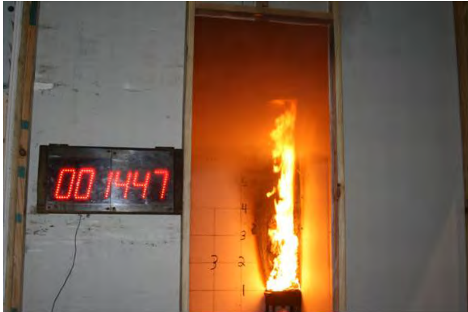
Figure 3. Burner at 160 kW: 14 min 47 s into Test.
